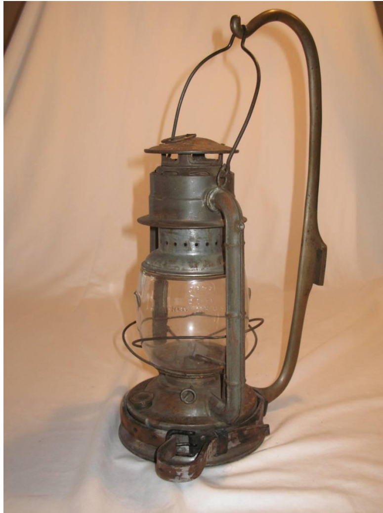
Dietz 'D-Lite' cold blast lantern, modified bail for Boston Fire Dept. Brass tag brazed to fount, reads "Lad. 31". Attached to custom BFD brass bracket, with hook and leather strap and brass buckle. Mounted on apparatus, circa 1910-1945. (Note: cold blast lanterns put out 10 candlepower, whereas fancy Dietz "King" F.D. lanterns were hot blast type, with only 4 candlepower.
